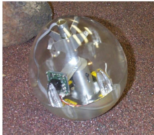
Figure 5: Testing configuration of the hopping robot.
