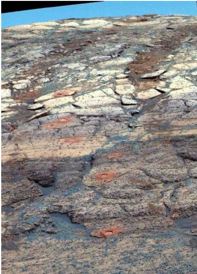
Figure 6: False color image taken on sol 173 showing RAT holes and rover tracks made during descent into Endurance.
