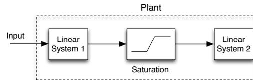
Fig. 2. Saturation sandwiched between two linear systems
