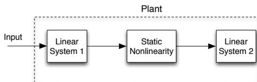
Fig. 1. Static nonlinearity sandwiched between two linear systems
