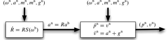
Fig. 2. Structure of system containing attitude, position, and velocity
