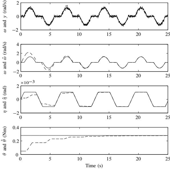
Fig. 1. From top: angular velocity  $\omega$  (solid) and noisy measurement  $y$  (dashed); angular velocity  $\omega$  (solid) and estimate  $\hat{\omega}$  (dashed); internal friction state  $\eta$  (solid) and estimate  $\hat{\eta}$  (dashed); unknown parameter  $\theta$  (solid) and parameter estimate  $\hat{\theta}$  (dashed)
