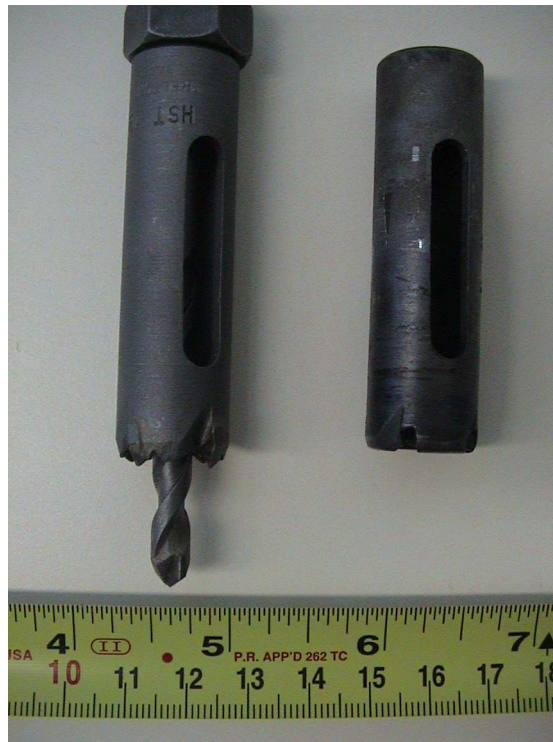
Figure 9: New Coring Bit with Centering Bit (left) and Worn Coring Bit without Centering Bit (right)
