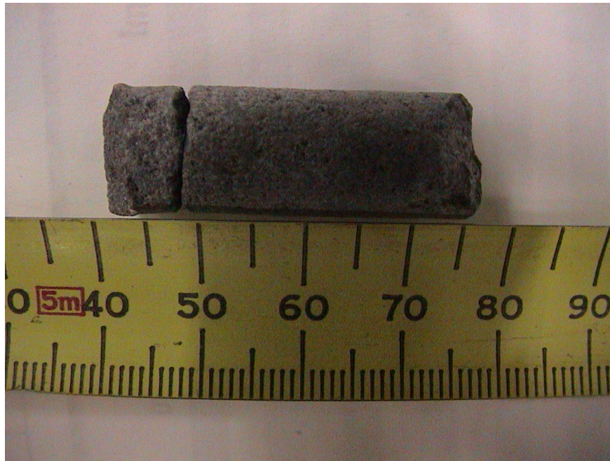
Figure 16: Intact Core Taken with No-tines Technique in Granite
