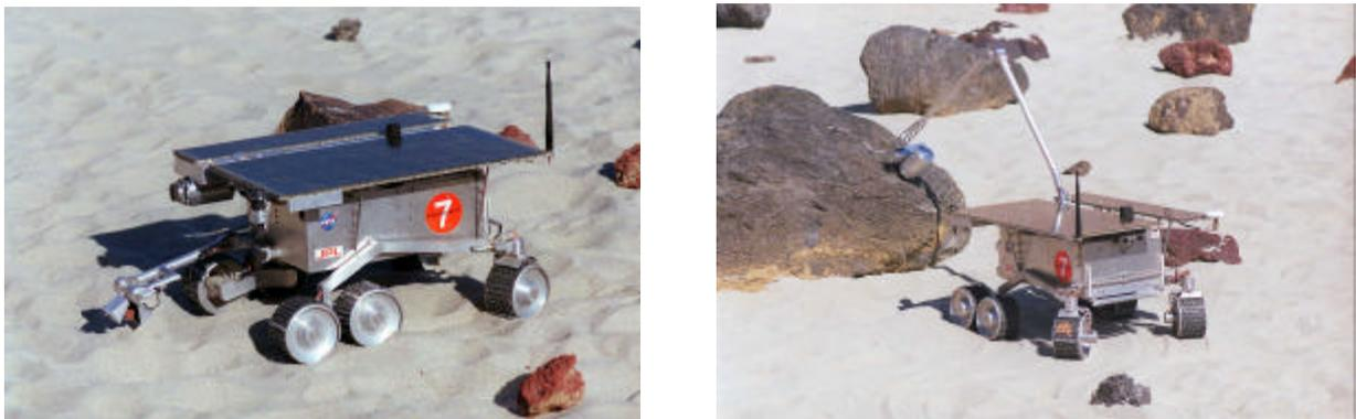
**Figure 10** The Rocky 7 rover completing the small rock acquisition (left) and the science instrument placement (right) procedure.
