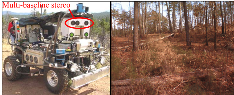
Fig. 16. The PerceptOR Raptor UGV was operated on a variety of terrain types, including forested terrain at Ft. A. P. Hill. A multi-baseline stereo system was used that could provide wide, mid, or narrow baseline stereo range data, depending upon how cluttered the scene was.
