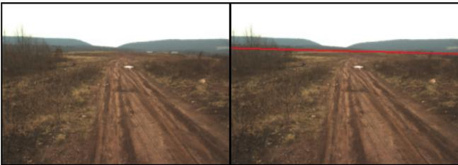
Fig. 4. A CAHV camera model and UGV attitude data from an onboard inertial measurement unit can be used to estimate the horizon line.
