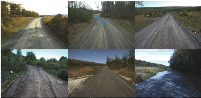
Fig. 17. Seven sequences of driving on cross-country trails were analyzed for false positive water detection using the sky reflection based detector with the false positive detection rejection algorithms enabled. Six are illustrated here and the seventh is illustrated in Fig. 14. In the 1711 frames processed over a 0.44km distance, false positive detection only occurred in 3 frames, a rate of 0.18%.
