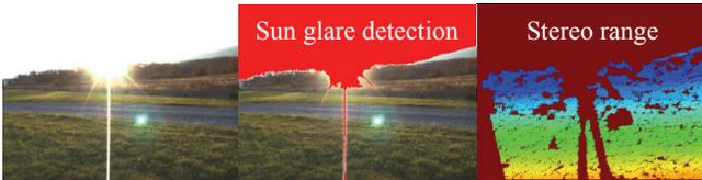
Fig. 11. When the sun is within the FOV, sun glare can occur, typified by a ray of saturated pixels extending from the sun to the bottom of the image. Sun glare causes lines of data loss in stereo range images. Water detection is not performed on images where sun glare is detected.
