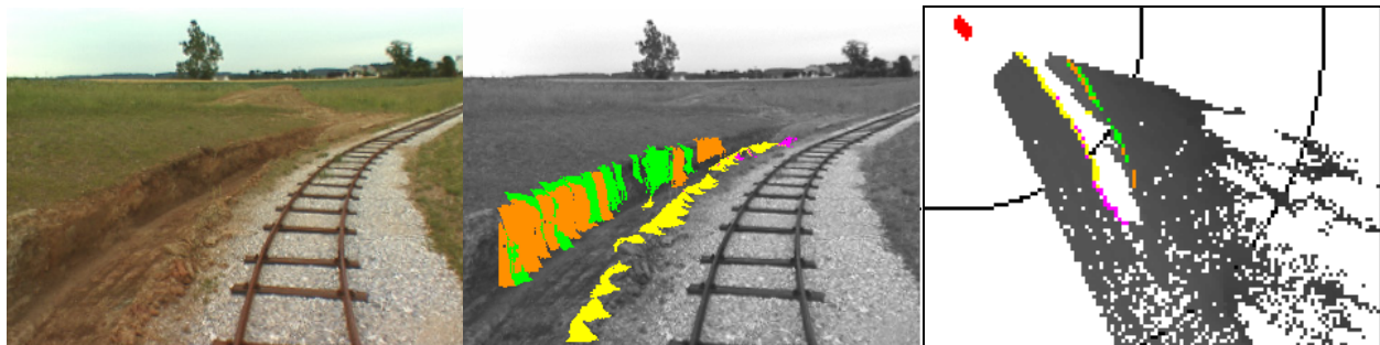
Figure 7. A frame showing a portion of the trench oriented parallel to the tracks (left), obstacle detection results overlaid on an intensity image (middle), and a north-oriented local terrain map (right). Multiple obstacle detectors locate different characteristics of the trench.
