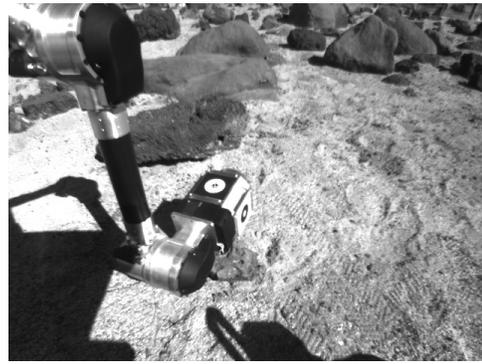
**Figure 16.** Final approach to target using image-based instrument placement. Tracking of the fiducial markers is done through the hazcams.
