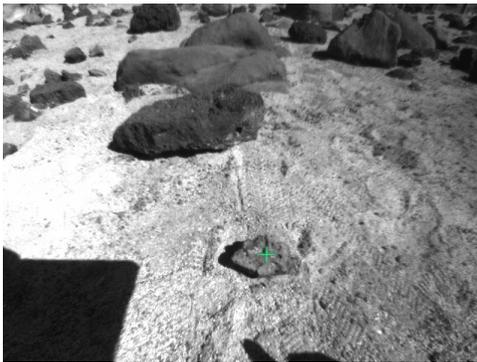
**Figure 15.** Target is retriangulated after achieving the location that maximizes arm manipulability.
