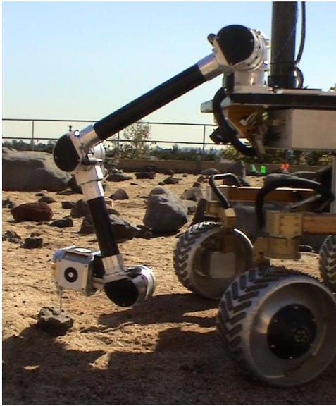
**Figure 11.** Rocky 8 5 DOF arm. Arm is deployed to place an instrument on a science target. Fiducial markers are mounted on the turret. These markers are used by HIPS to accurately position the instrument on the target. Front hazcams are shown mounted below the deck.
