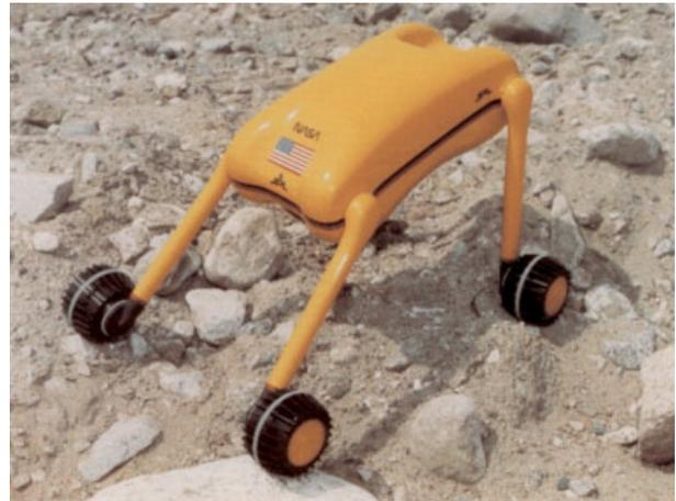
**Figure 2.** GoFor (1992)—High mobility robot vehicle developed by Brian Wilcox, with wheels-on-legs configuration, able to climb vertical steps of height 70% of the maximum stowed vehicle dimension.
