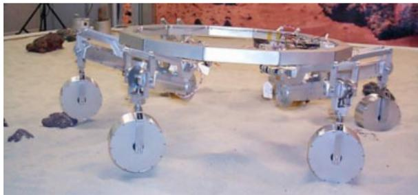
**Figure 3.** Prior wheel-on-leg vehicle with six wheels in symmetric hexagonal array, able to climb steps 50% of max stowed vehicle dimension.
