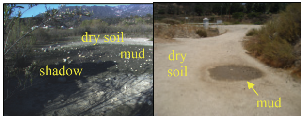
Figure 2. Mud tends to be darker than surrounding dry soil in color imagery.
