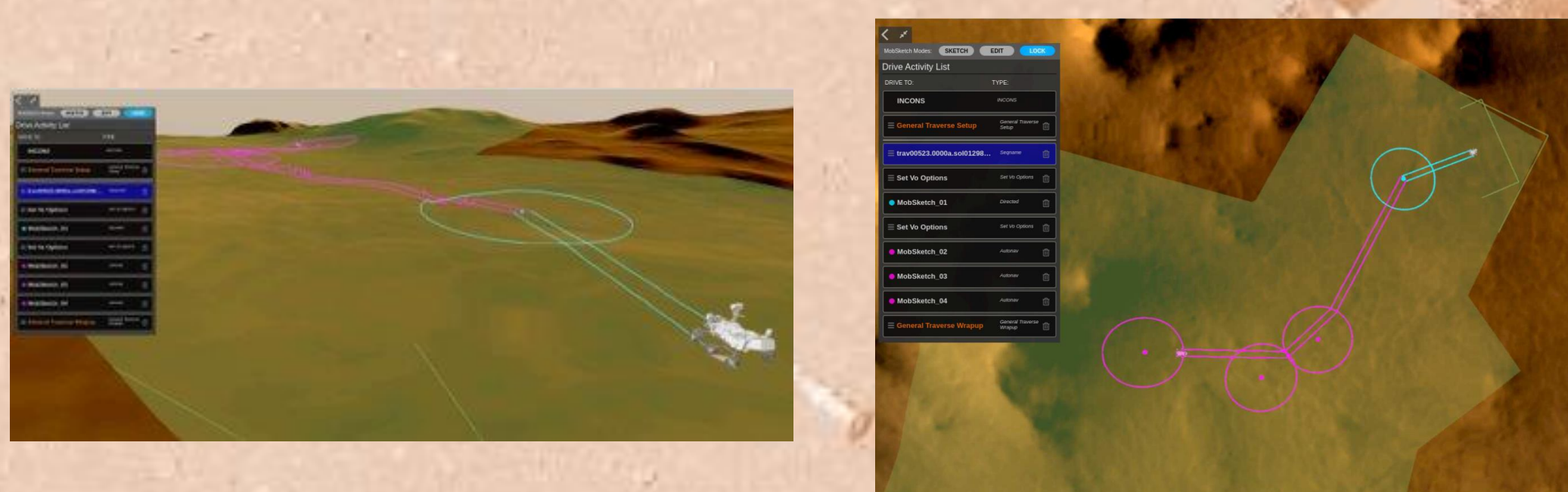
Figure 1. MobSketch planning tool showing Perseverance ascent of Jezero Crater rim (sol 1296, Oct 2024), the first use of AutoNav at >20^\circ tilt. Light blue: DIRECTED drive, Pink: AUTONAV drive, Light green: keep-in zones, Black reference box summarizes drive segments and other commands. Graphical drive plans are expanded automatically into hundreds of rover commands in < 1 second after each change.
