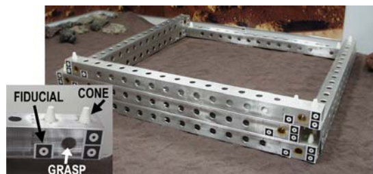
Fig. 1 The structure of interlocking beams. Inset: Component end with three fiducials and two interlocking cones
