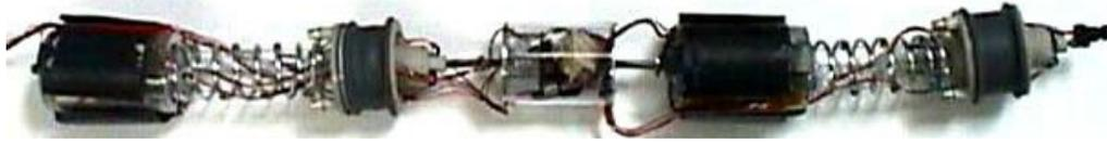
**Figure 13** An in-pipe robot built by JPL for natural gas pipelines. The prototype uses airbags to push against the inside of the pipe. The robot moves with an inchworm motion and uses a three degree of freedom joint between segments to navigate elbows and tees. A propeller harvests energy for the robot from flow in the pipe.
