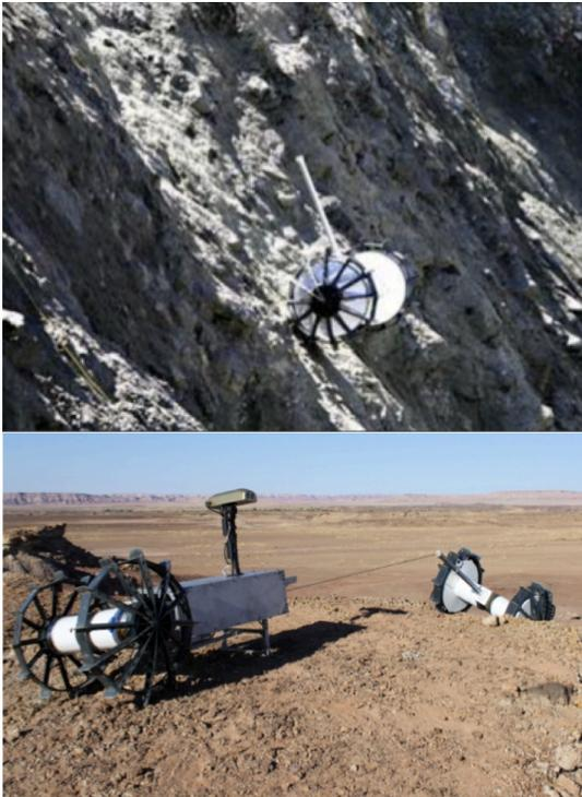
**Figure 11** The Axel rover descending a steep cliff face (top). Axel undocks from the DuAxel and repels down the cliff using a tether (bottom).
