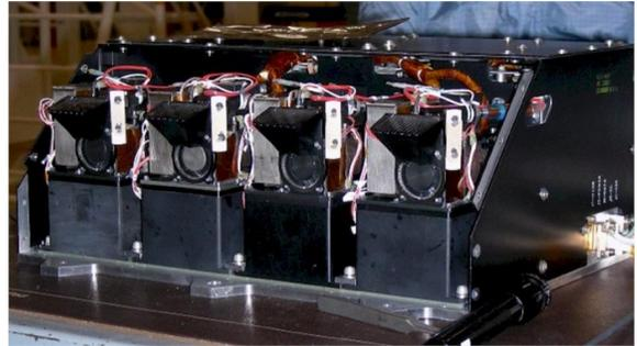
**Figure 1 Phoenix mission Microscopy Electrochemistry and Conductivity Analyzer (MECA) instrument with the Wet Chemistry Laboratory (WCL) beakers displayed (Hecht, 2009).**
