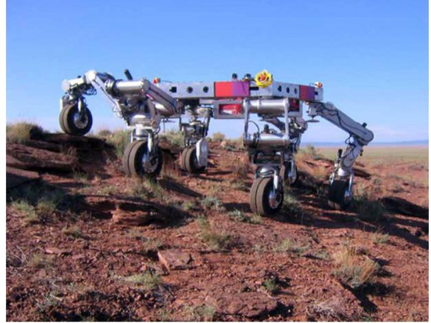
**Figure 9** The ATHLETE rover is a highly capable multi-modal mobile robot. By combining the rough surface performance of legged robots with the efficiency of wheeled driving, ATHLETE is able to move quickly and efficiently across a broad range of terrain. The limbs can also function as manipulators with a variety of tools to do maintenance tasks.
