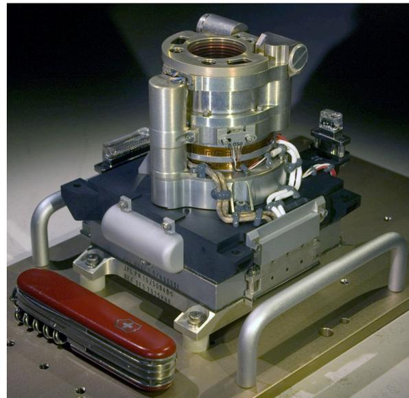
**Fig. 1.** The flight MAHLI camera head with pocket knife (88.9 mm long) for scale.
