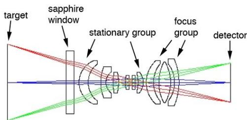
**Fig. 2.** MAHLI optics diagram, with ray traces.
