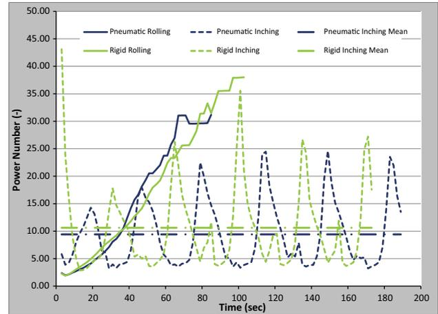
Fig. 12. Power number (total power consumed normalized by vehicle weight and velocity).
