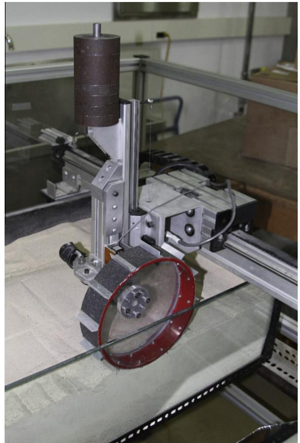
Fig. 2. Wheel test rig used with Soil Optical Flow Technique.
