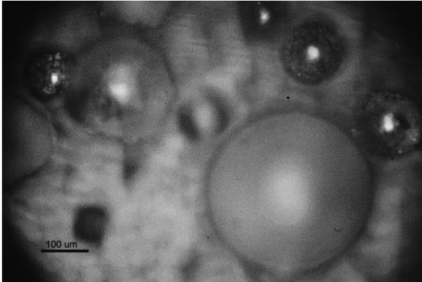
Fig. 5. View of Fillite microspheres under microscope (100× magnification).
