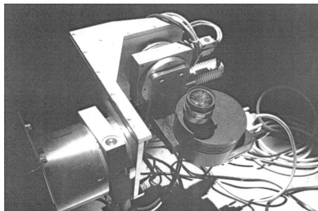
Fig. 4 Sun-illuminated lens mounted in goniometer.
