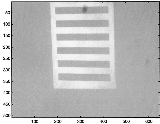
Fig. 7 Image of the bar target. Sun illuminates the dust-contaminated lens front surface. The dust contamination level is 46% transmission relative to no contamination.
