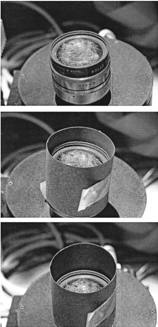
**Fig. 10** Dusty lens with different length sunshade.
