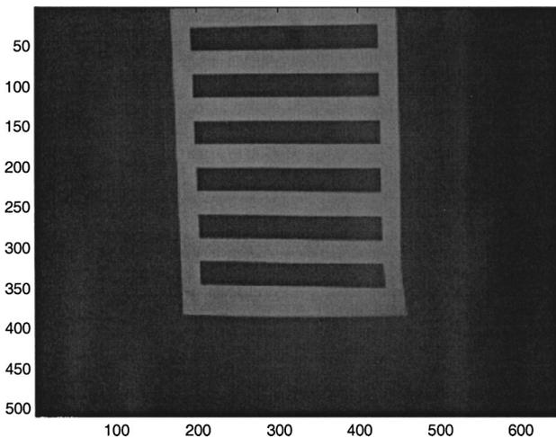
Fig. 6 Image of the bar target. The sun does not hit the dust-contaminated lens front surface. The dust contamination level is 46% transmission relative to no contamination.
