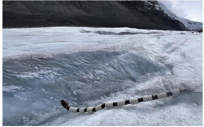
**Figure 7:** EELS 1.0 descending into the AC2 channel in Surface Test 3 on Day 14
