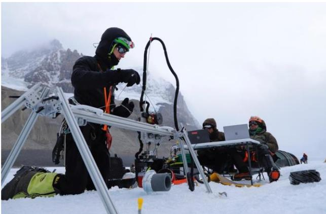
**Figure 16.** Field-deployable screw mobility testbed on a horizontal surface ice near the Base Camp.
