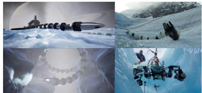
**Figure 1:** Left - Mission concept illustration of the EELS robot traversing on the surface of an icy moon (top) and descending into a vertical conduit (bottom). Right - EELS 1.0 (top) and EELS 1.5 (bottom) prototype robots conducting mobility trials on the Athabasca Glacier, a terrestrial icy-moon analog. Credit: NASA JPL.
