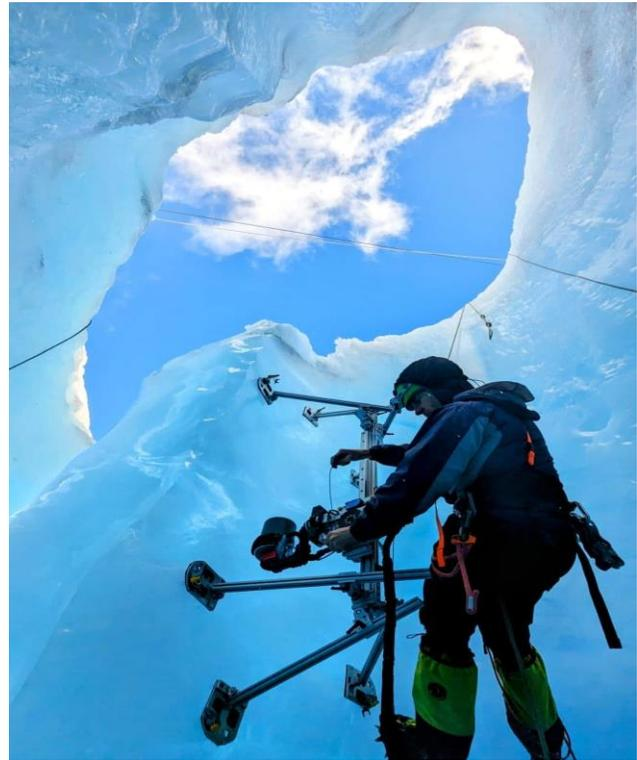
**Figure 17.** Field deployable screw mobility testbed on a vertical wall (blue ice) in the M8 moulin
