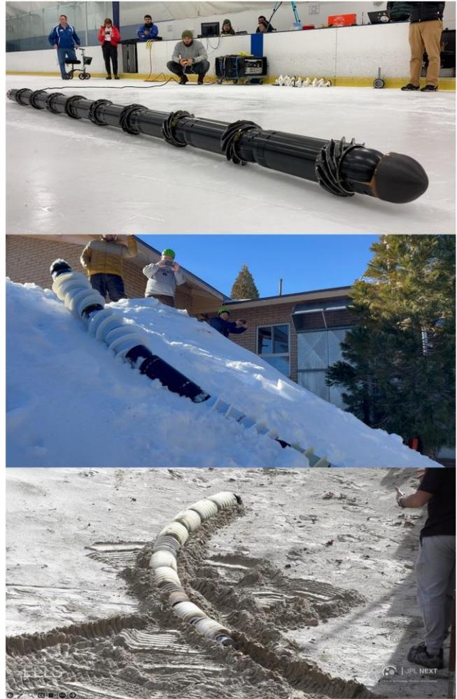
**Figure 2;** Surface mobility tests of the EELS 1.0 prototype robot on an ice rink (*top*), on loose snow (*middle*), and on loose sand (*bottom*). Credit: NASA JPL
