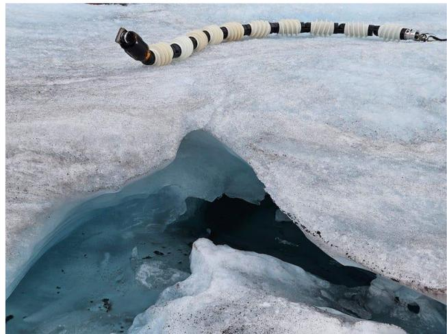
**Figure 8:** EELS 1.0 avoided a negative obstacle semi-autonomously in Surface Test 4 on Day 15.
