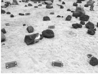
Figure 21. Bricks with reflective targets were used for stereo range error measurements
