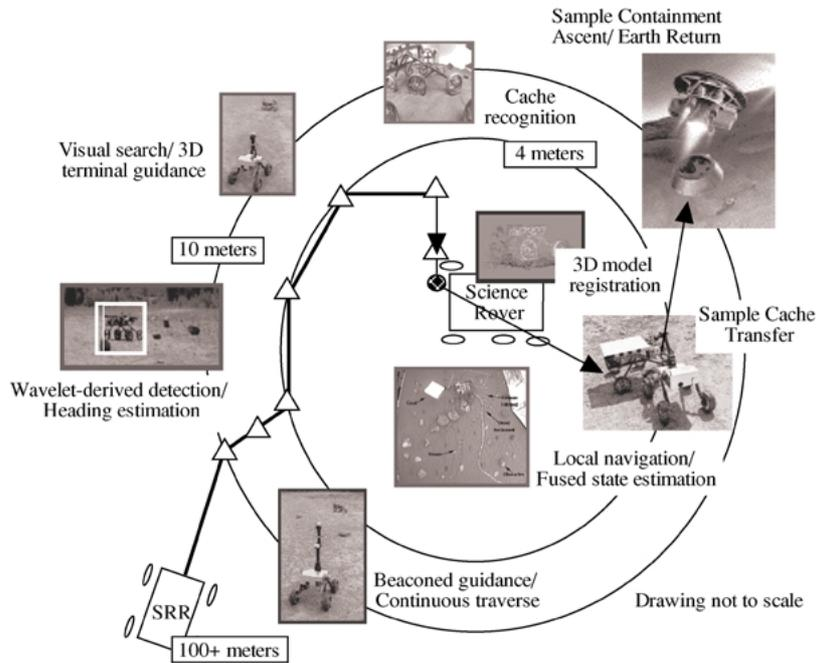
Figure 6. Rover-to-rover rendezvous, sample cache retrieval in early SRR field testing at Arroyo Seco near JPL.
