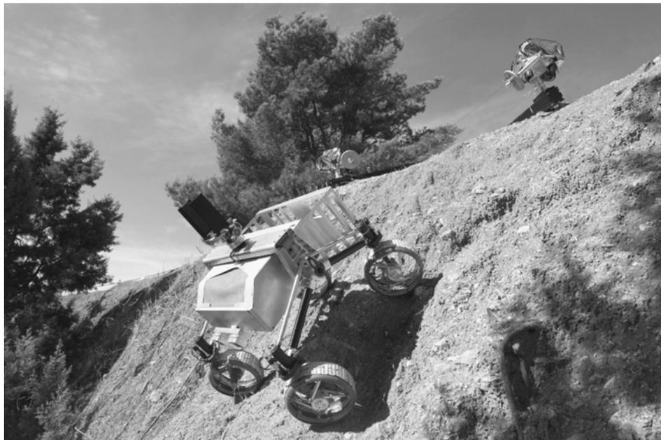
Figure 21. Cliff-bot performing active way point navigation on a cliff face with closely coordinated active tether control by two anchor-bots at the top of the cliff.
