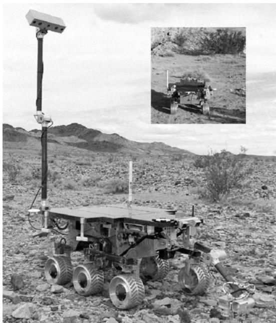
Figure 1. FIDO Rover in desert field test on a cobbled lake bed, mast/science arm extended (inset, rover continuously traverses a sand wash, rear view, the mast/arm stowed (Weisbin et al., 1999)).
