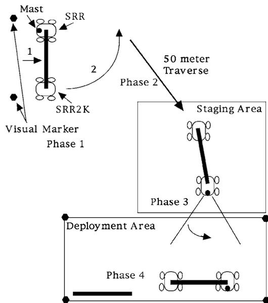
Figure 18. (1) Initiate transport configuration, (2) move to staging area, (3) initiate site survey, and (4) dock into site.
