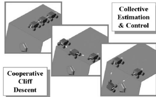
Figure 19. Multiple, modular robots reconfigure to perform a cooperative descent for analysis of cliff stratigraphy.
