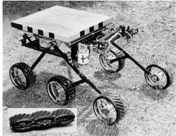
Figure 5. Lightweight Survivable Rover (LSR), with rear-mounted sampling arm, driven by rotary ultrasonic motors (Schenker et al., 1997). The arm carries an opposable gripper, rock abradar, and color micro-imager. The affixed "can" is a simulated sample container. The 20 cm dia. wheels are collapsible (*inset*) and self-deploying on compression release. LSR carries a front-mounted, multi-spectral science imager.
