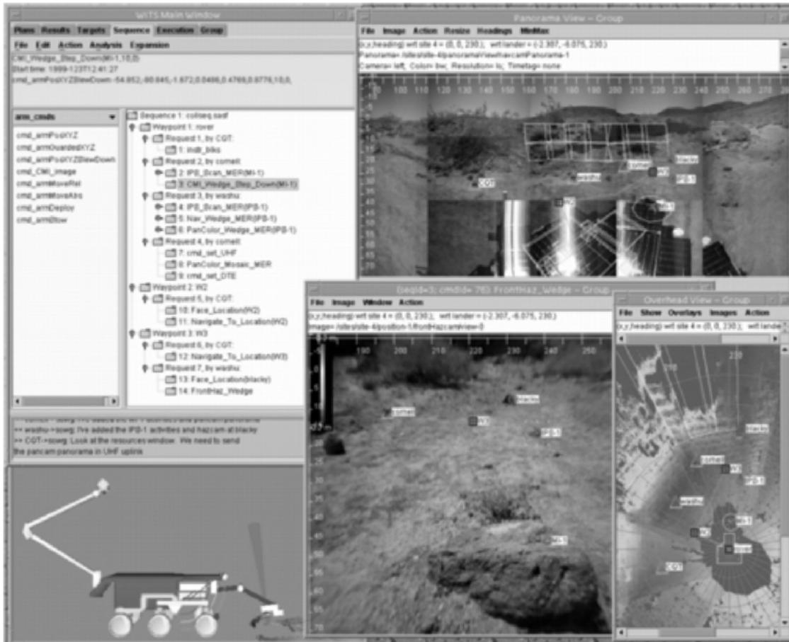
Figure 2. Web Interface for Telescence (WITS) display as seen by a single operator at a PC/Unix-based workstation.
