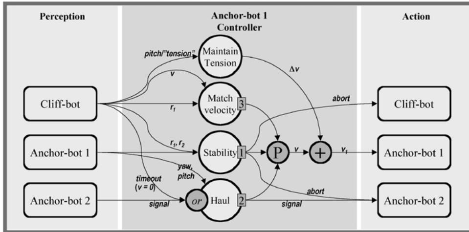
Figure 20. A subset of the behavior network for collective cliff-descent illustrating sub-system for controlling the velocity of anchor-bot 1. The arrows represent data links between local blocks as well as remote components (behaviors, sensors, actuators) thus spanning a behavior network across the team of robots.
