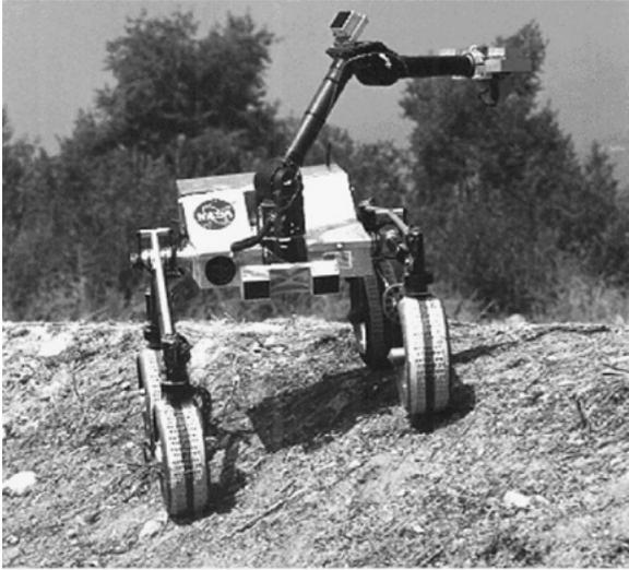
Figure 12. SRR in steep descent on hill at Arroyo Seco near JPL. By comparison to a fixed geometry and nominal c.g. (arm stowage position), rover tip-over instability is greatly improved.
