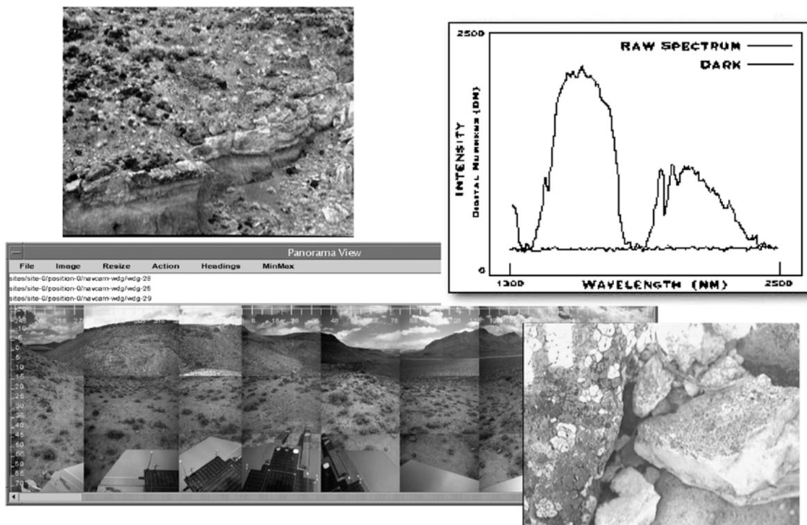
Figure 4. Representative data products from FIDO Rover field test at the Nevada. Upper left, near-field Panoramic Camera sector; lower left, Navigational Camera mosaic; upper right, Infrared Point Spectrometer analysis of target; lower right, close-up of ground rock structure taken with micro-imager. See also <http://wufs.wustl.edu/fido>.
