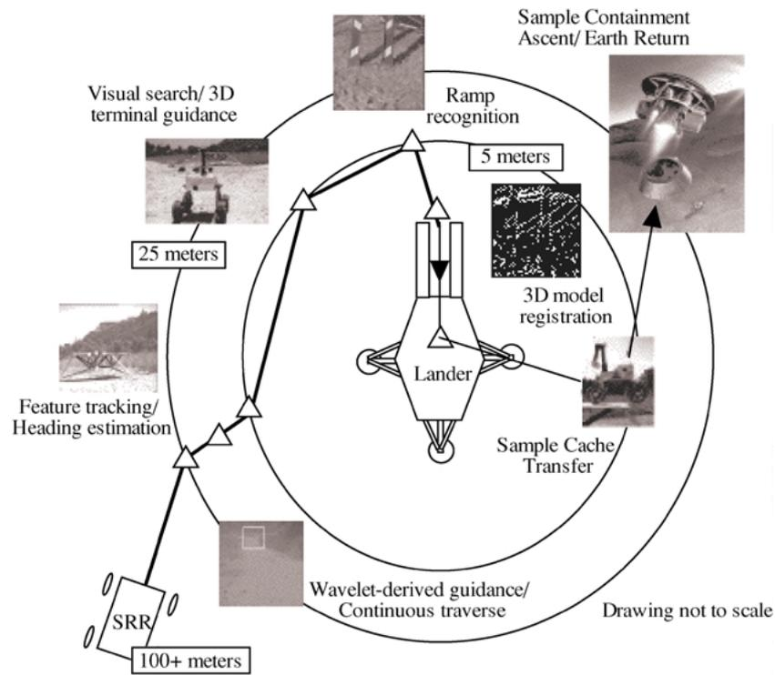
Figure 8. Rover-to-lander visual rendezvous for sample return cache transfer, performed at Arroyo Seco near JPL.
