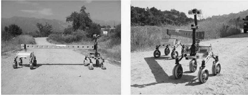
Figure 16. Coordinated transport of extended container (2.5 meters) by SRR and SRR2K, as performed in Arroyo Seco near JPL. (Left) row transport formation; (Right): column (leader-follower) transport formation.
