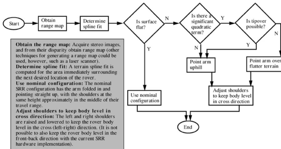
Figure 11. Simple control adaptation scheme for the SRR reconfiguration in response to perceived terrain model.
