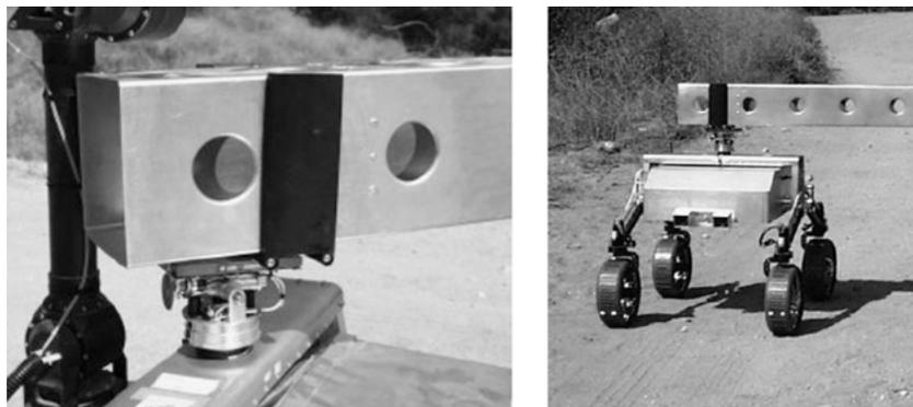
Figure 17. Instrumented gimbal (SRR2K close-up at left).
