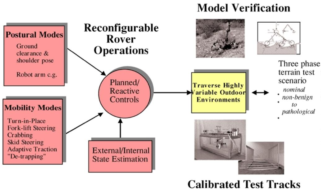
Figure 10. Experimental concept for development and test of SRR reconfigurable control over adverse terrain.
