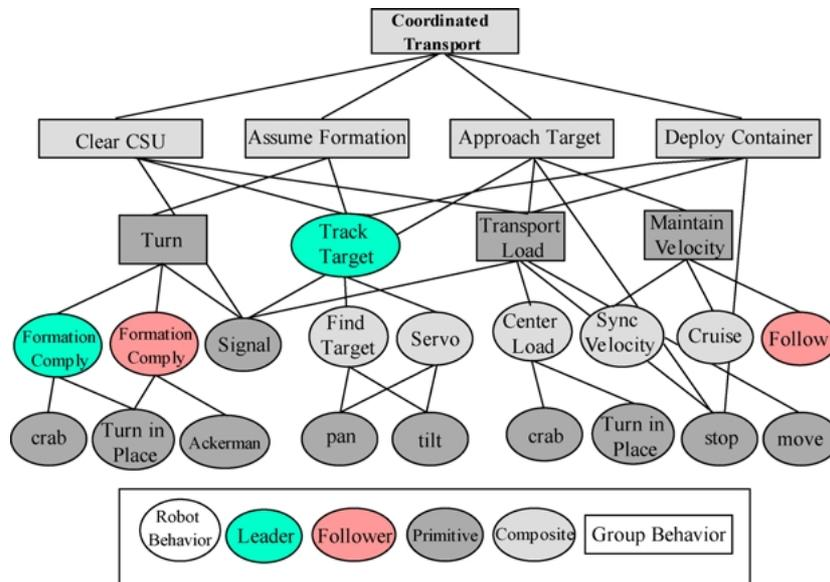
Figure 15. CAMPOUT “behavior hierarchy” describing a coordinated transport task (see Fig. 13, frame 2, graphic). Bubbles represent single robot behaviors; boxes represent multi-robot “group” coordinated behaviors. Higher-level actions, themselves behaviors, are composed from yet lower-level behaviors (Pirjanian et al., 2000).
