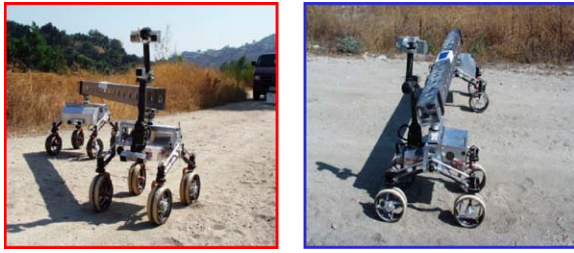
Figure 5. Transport formations for the Robot Work Crew (SRR in foreground and SRR2K in background): (left) Column formation for transport and obstacle avoidance; (right) Row formation for precision placement.
