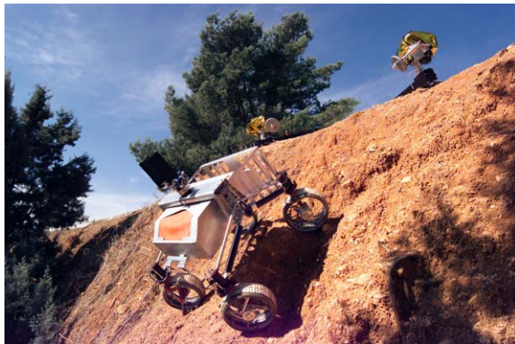
Figure 1. Cliff-bot performing active way point navigation on a cliff face with closely coordinated active tether control by two anchor-bots at the top of the cliff.
