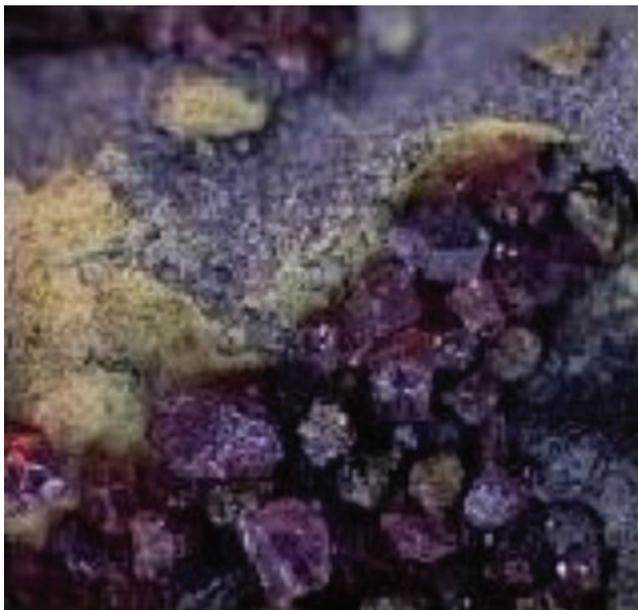
**Figure 16.** A Microscopic Imager (MI) view of garnet sand in FIDO's indoor testing sandbox.
