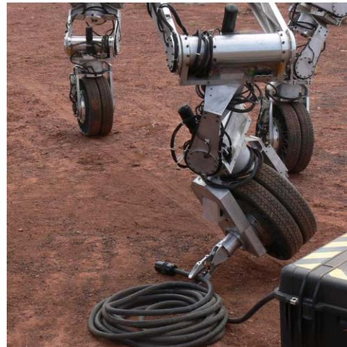
**Figure 9. Gripper attached to ATHLETE limb shown manipulating a cable**
