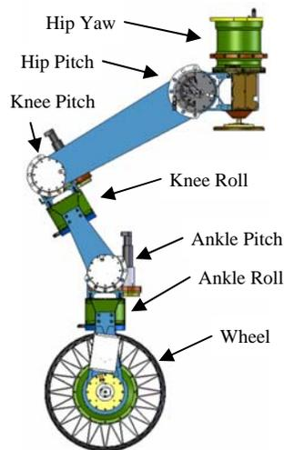
Figure 2, Kinematic layout of the limb.
