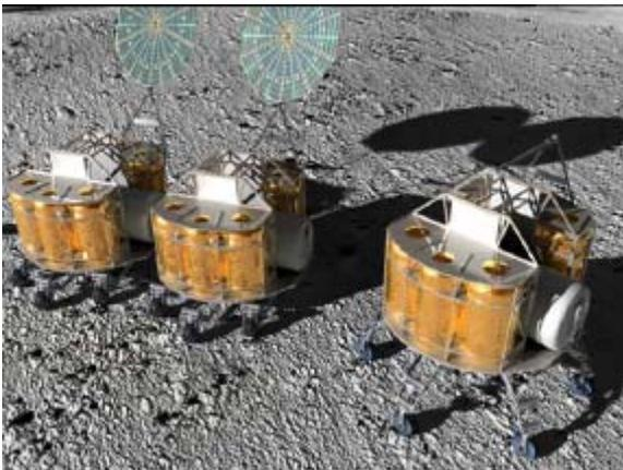
**Figure 13, ATHLETE vehicles shown carrying pressurized crew compartments in an artist's concept. Image courtesy of NASA Langley Research Center.**
