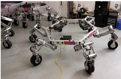
**Figure 3, The hexagonal body of the ATHLETE vehicle with limbs at each vertex**
