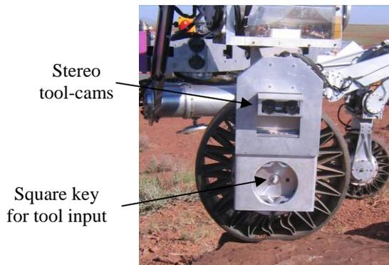
**Figure 8. Tool mechanism located at the end of each ATHLETE limb**
