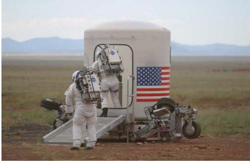
**Figure 10, Suited astronauts entering a simulated pressurized rover compartment on the deck of a squatted ATHLETE vehicle**
