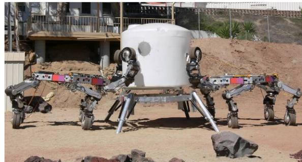
**Figure 12, Two ATHLETE vehicles shown lifting a mock pressurized crew compartment from a mock lander.**
