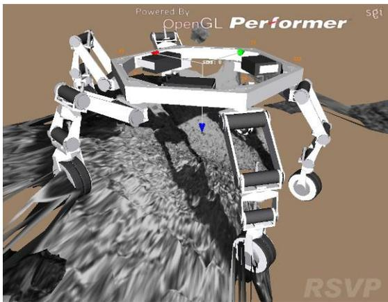
**Figure 7, Terrain mesh showing 3-D environment around the vehicle constructed from stereo imagery**
