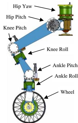
Figure 2, Kinematic layout of the limb.
