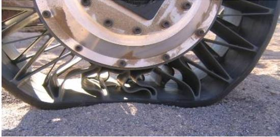
**Figure 5, An ATHLETE Tweel<sup>™</sup> shown deforming over uneven terrain**
