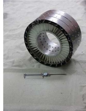
**Figure 6: The Lunar Tweel Prototype and the resulting uniform contact patch in soft soil after applying 100kgs.**
