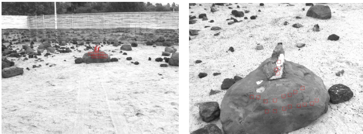
Figure 8. Tracking with straightforward rover motions. Targets were about 10 m away from the rover in the initial image (left), and about 2.3 m away in the final image (right). The image sequence was collected in 30 rover step motions from an actual on-line run. Target windows resulting from 20 off-line tracker runs were overlaid.
