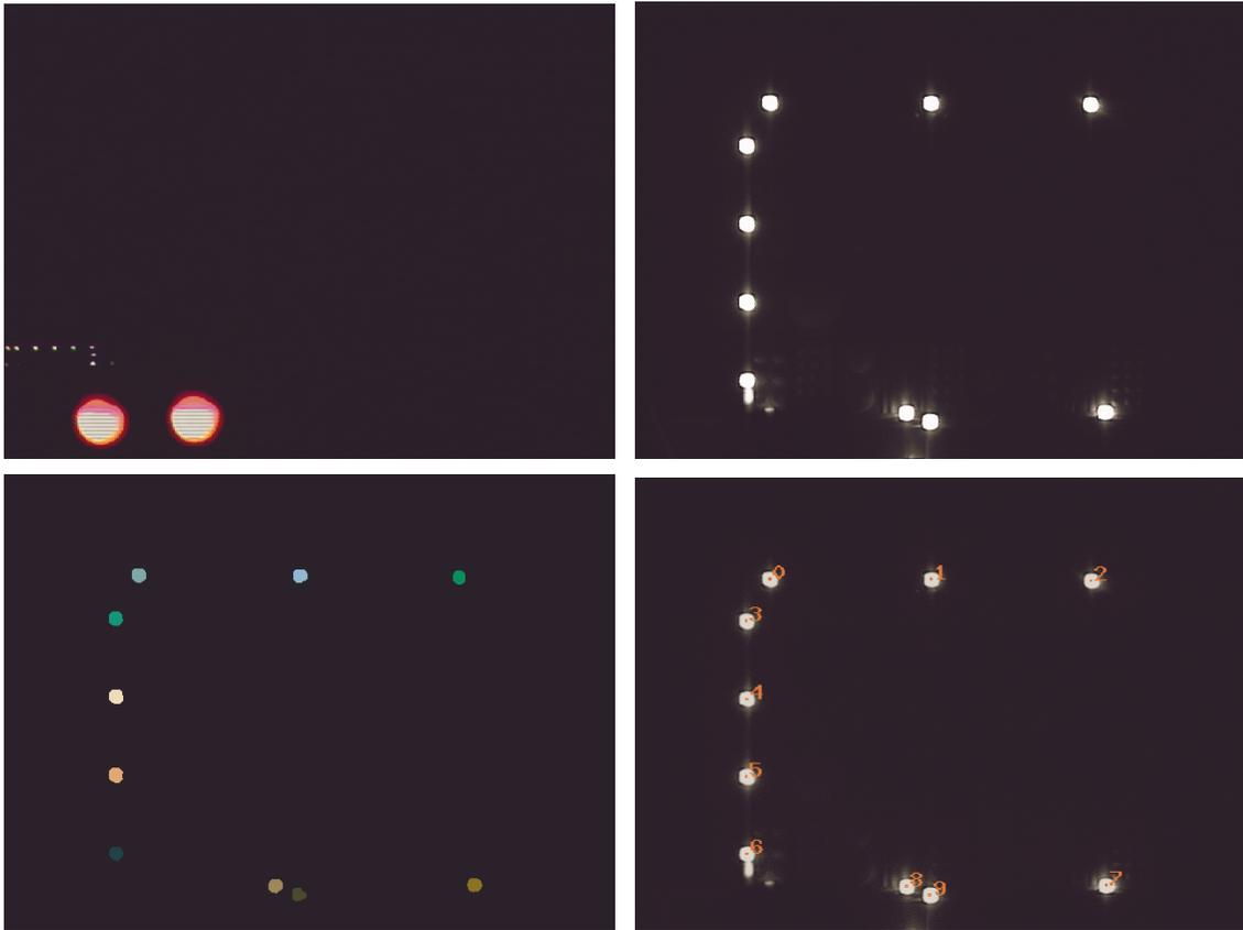
**Figure 8 Digicam images used to estimate sled attitude. (top left) The LED image with lights in background. (top right) Example light input image. (bottom left) Connected components extracted from light image. (bottom right) Labeled centroids of lights.**
