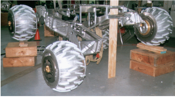
Fig. 4: Nomad chassis showing averaging effect of bogies
