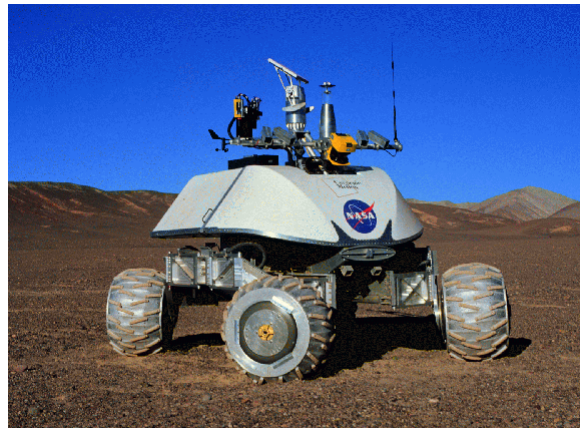
Fig. 3: Nomad with wheels positioned for turning in place the wheels must be steered to an extreme, 49^\circ , before pivoting. The preferred mode of steering for Nomad is double Ackerman. Most automobiles have Ackerman steering on the front wheels; Nomad can steer its front and rear pairs. Just like a car, when turning, the wheels pivot by different amounts, because their distances to the center of turning are not the same. Nomad accomplishes this with two pairs of four-bar linkages—one pair on each side. A push-rod is attached to one axis of each linkage and is driven by two racks which are pulled in opposite directions by a single pinion placed between the two linkages. This pivots the front and rear wheel of each bogey by an equal but opposite amount.
