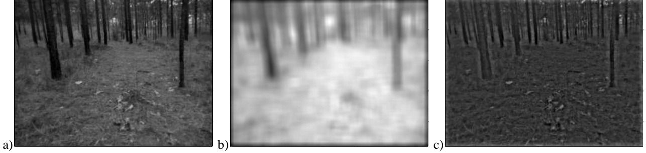
Figure 1: a) Image of outdoor scene. b) Averaging with 15x15 filter. c) Background subtracted image. Note the ringing artifact around the trees.
