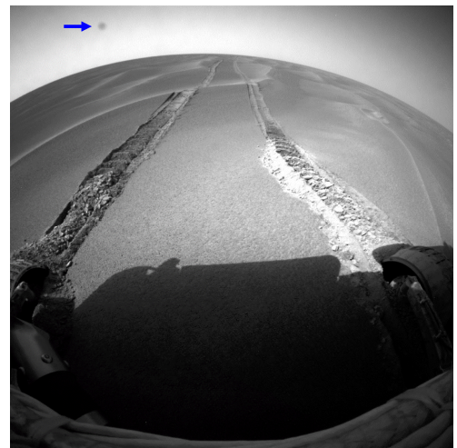
Fig. 23. Opportunity right front Hazcam on Sol 471 after dust contamination.
