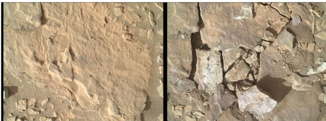
**Figure 14.** Before and after 40 cm standoff WATSON images of the Chiniak abrasion attempted on sol 562. Note the significant rock fracturing and changes in surface topography due to the abrasion operation. Credit NASA/JPL/Malin Space Science Systems.
