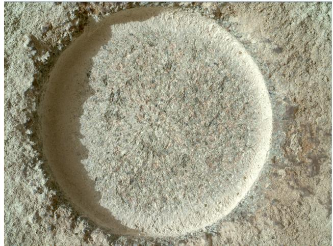
**Figure 18.** Eremita Mesa abrasion patch from sol 1257, following gDRT puffs. The gDRT was used to clear dust from the exposed rock surface after the abrasion process, enabling proximity science instruments PIXL and SHERLOC to analyze the freshly revealed, unweathered rock beneath the Martian surface layer.
