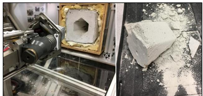
**Figure 22. Shown is an acquired sample of a 5.2MPa CPR MPACS simulant block from the Rigid Testbed. The hole created reached 15cm depth and acquired a mostly intact 520cc volume sample. The blade end of travel velocity was 5.5m/s (at full blade closure). Four tests ranging from 5.2 to 5.6 MPa CPR were repeated with similar results.**
