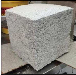
**Figure 17. Mechanical Porous Ambient Comet Simulant (MPACS) simulant block.**
