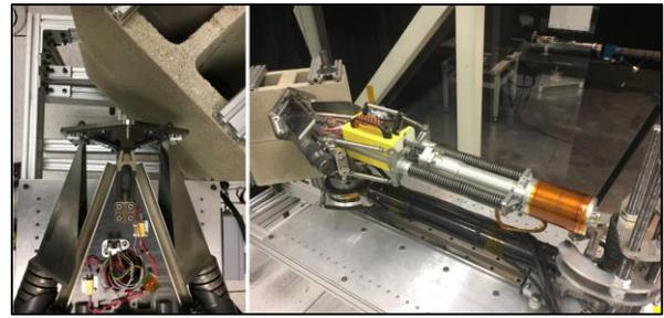
**Figure 29. Validation testing of energy transferred to S/C during rigid surface oblique strike scenario. Shown is a rigid, smooth surface (cinder block) fixed at 45° to the BiBlade sampling axis with the face of the sampler touching. This configuration represents the worst-case scenario for blade interaction with a surface that may lead to excessive spacecraft rotational rate.**
