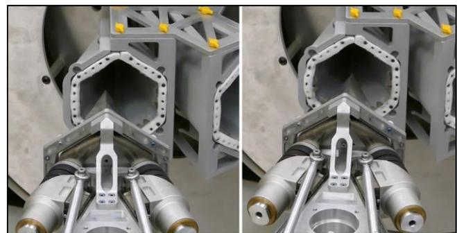
**Figure 25. Validation of robustness to robotic arm misalignment during insertion of BiBlade into SRC vault. Linear and angular offsets were introduced and proper lid deployment and capture was verified. A 4cm transverse offset (left figure) and 5° angular offset (right figure) are shown to have no adverse effects on sample transfer.**
