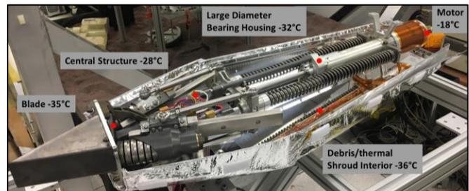
**Figure 32. Temperature of critical components during cold/vacuum operation testing with  $-160^{\circ}\text{C}$  cold shroud. Measured temperatures (see red dots for locations) were consistent with component allowable temperature limits and requirement of sampling surfaces (blade) to maintain temperature below  $-25^{\circ}\text{C}$ .**
