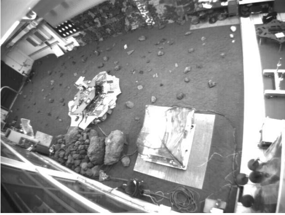
Figure 1: Sandbox as viewed by one of the cameras. Note the rover left of center, with target dots on solar panels, sitting on mock lander amidst much visual clutter.
