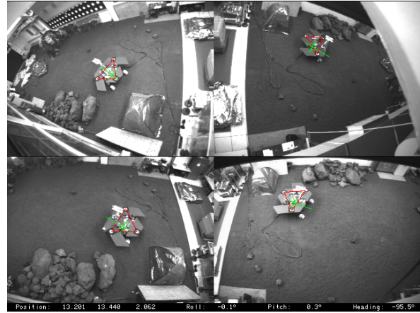
Figure 2: Display of tracker in action, as viewed by four different cameras. Red lines connect projections of located dot positions. Green lines form coordinate axes with elongation in the forward direction.
