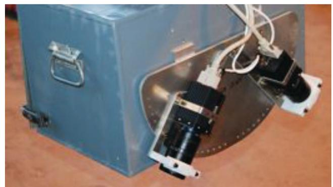
**Figure 4: Passive optical TRN cameras**
