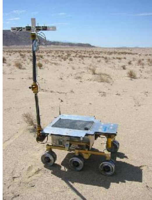
Figure 7: The Rocky 8 rover with the mast unstowed
