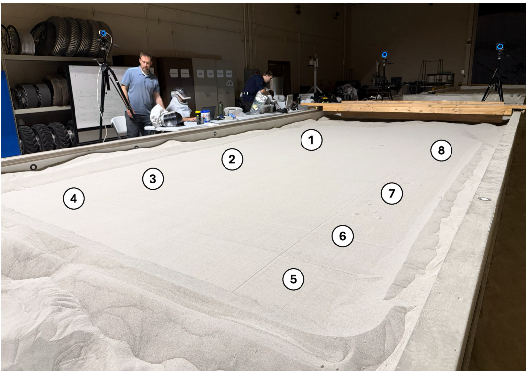
Figure 17. Fillite simulant testbed, in prepared state. Numbers indicate approximate locations of the cone penetrometer measurements detailed in Section 3.2.3.
