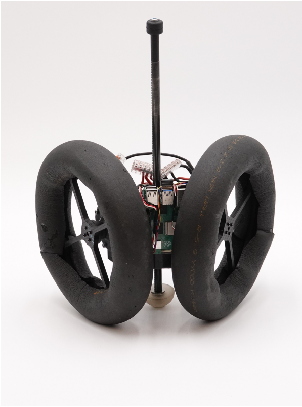
Figure 23. LEAP-S1 platform used for testing of jumping on granular media. Dual reaction wheels keep the platform balanced on the ground and oriented in the air. A single rack and pinion is used to drive the leg to jump and hop of varying terrain.
