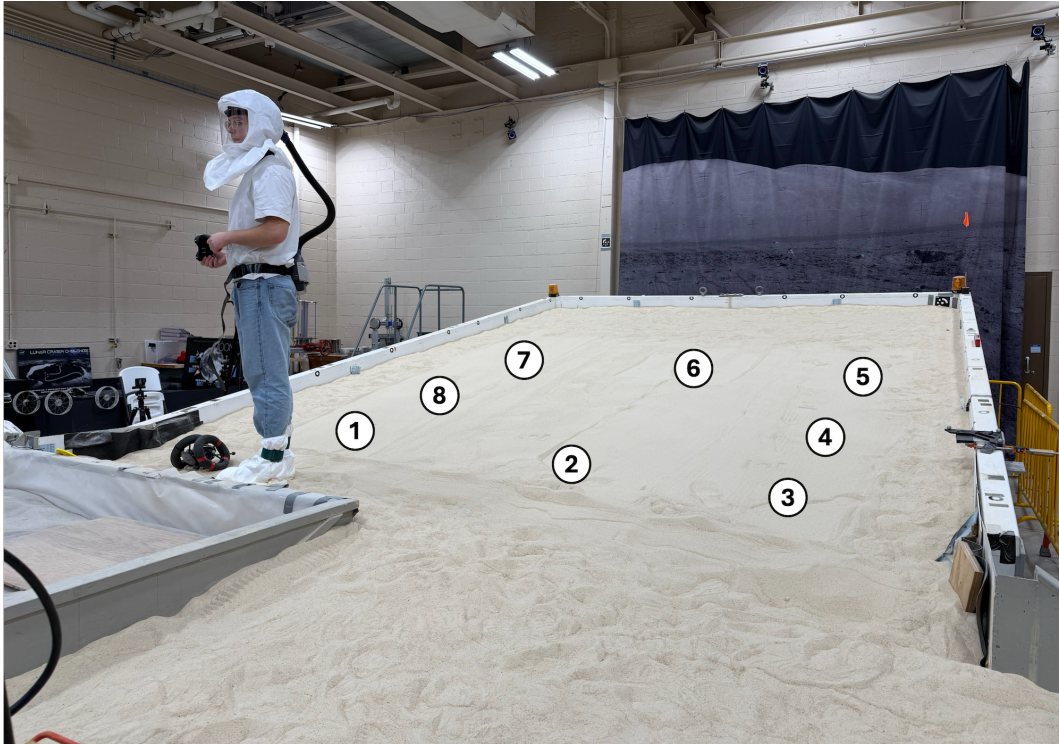
Figure 16. GRC-1 simulant testbed, in loose prepared state at a tilt of 10 deg. Numbers indicate approximate locations of the cone penetrometer measurements detailed in Section 3.2.3.
