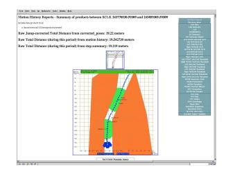
Fig. 2. Part of the Mobility/IDD HTML page summarizing Spirit's Sol 1323 Drive data. All data can be viewed at once, or a green pull-down menu can be used to limit attention to a particular class of downlink data. The course plot in the middle includes an auto-generated imagemap that provides hyperlinks to pages describing each individual plot point showing *all* data collected at that position.
