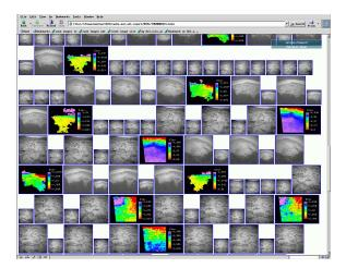
Fig. 3. Some of the A-1323 thumbnails included on the auto-generated HTML pages. Color annotations are elevation plots, computed on the ground by running stereo vision software on the 128x128 low-resolution images.
