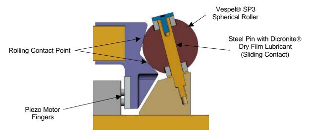
Figure 12. Spherical Roller Cross Section
