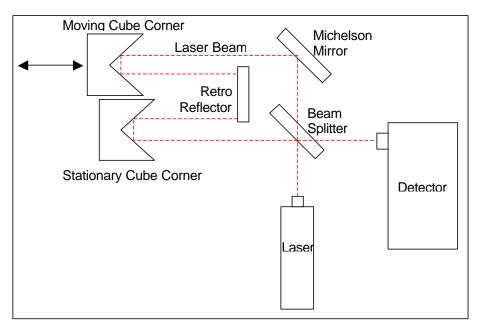
Figure 13. Laser Interferometer Test Setup
