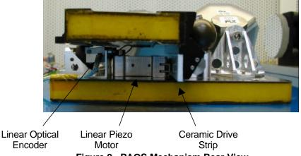
Figure 9. PAOS Mechanism Rear View
