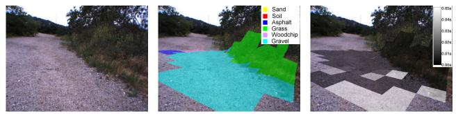
Figure 7. Experiment 2. Input color image (left), terrain classification results of the hierarchical classifier in a frame (middle) and the amount of computations performed on each cell (right) overlayed on the original image. The algorithm gains speed advantage from classifying some patches at close range with much less computation than the baseline method. Gravel terrain.
